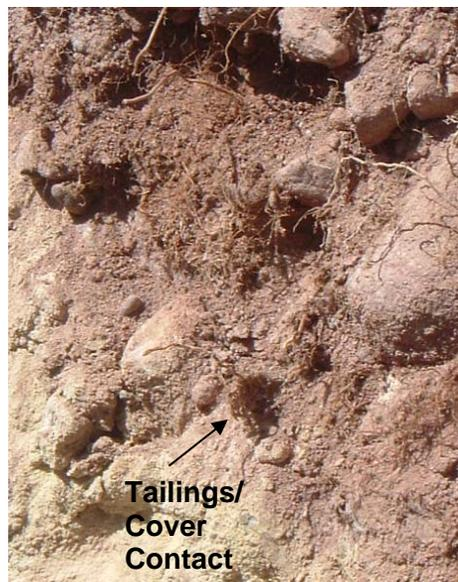
Figure 3. Matted roots in Tailings 4W 60 cm cover material
