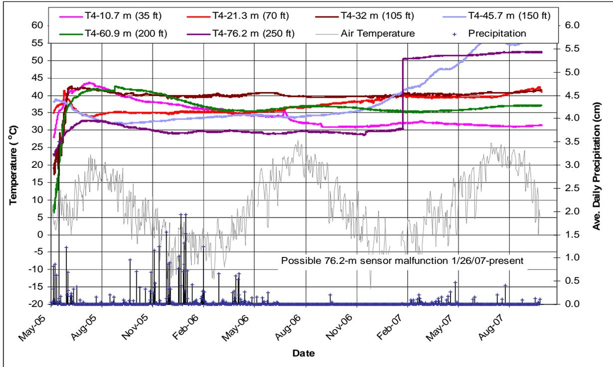
Figure 4. DAR-4: Temperature over time, by depth
