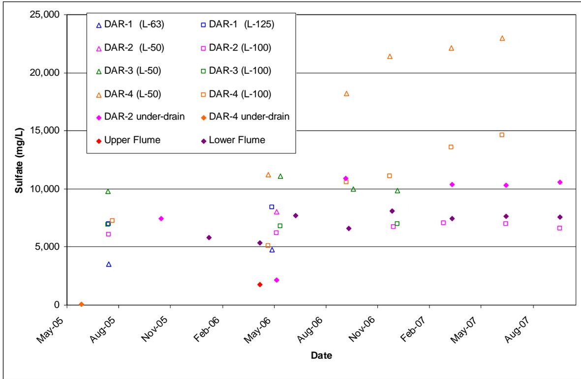
Figure 9. Sulfate levels in lysimeter and under-drain water samples over time
