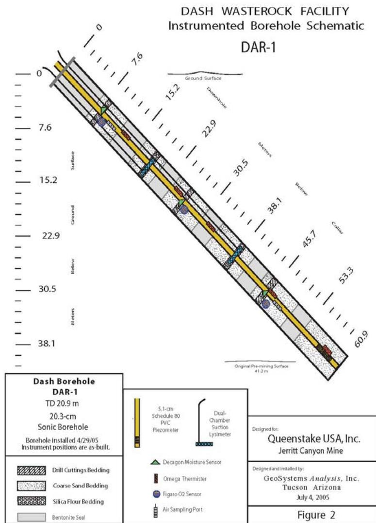
The four boreholes were located and constructed as follows:
