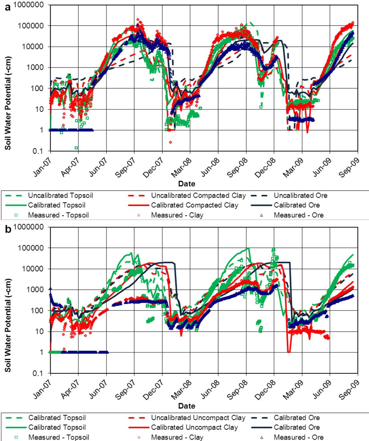
Figure 2. Model predicted and measured soil water potentials for (a) the compacted clay panel, and (b) the uncompact clay panel.
