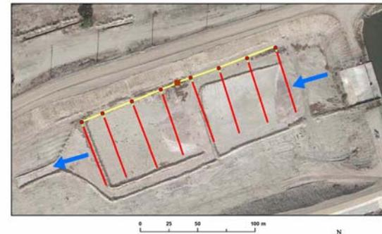
Figure 5. Pilot-scale riverbed filtration system.
