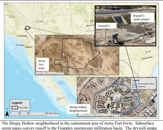
and sedimentation chambers are embedded in the infiltration basin.
