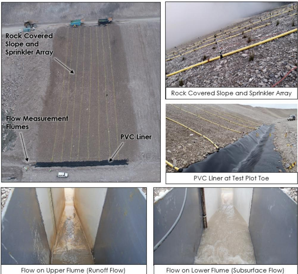
Figure 2 Test Plot Constructed to Simulate Runoff Response on Rock Covered Surface.
