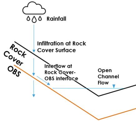
Figure 3 Illustration of Conceptual Model for UWOBs Rainfall Runoff.
