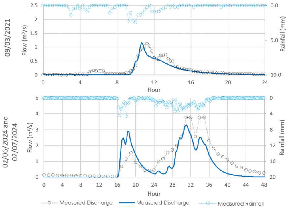
Figure 6 Stormwater Runoff Model Calibration Results during Rainfall Events in 2021 and 2024.
