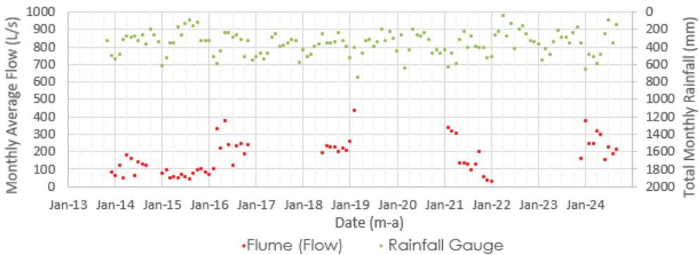
Figure 4 Record of Average Monthly Flow Rate (Flume) and Monthly Total Rainfall Depths (Rainfall Gauge).
